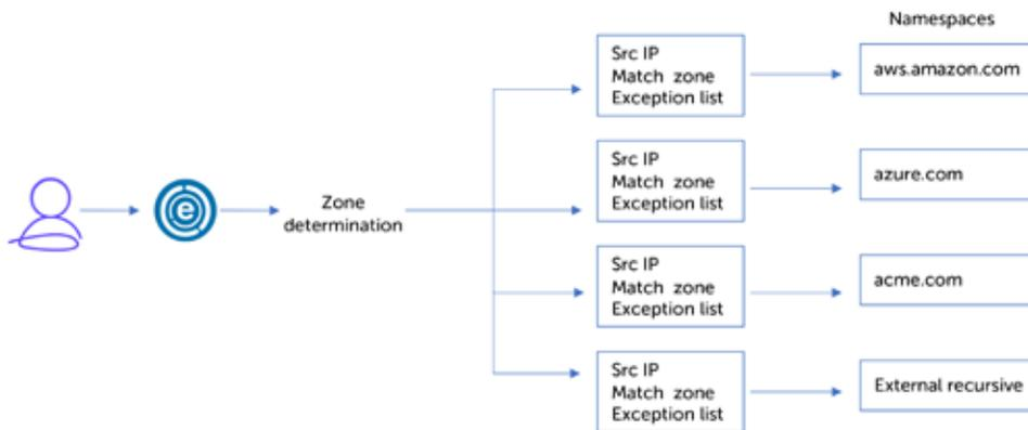
The above diagram shows a customer that has resources in AWS and Azure both while having a domain called acme.com. If none of the queries match then it will forward to an external resolver.
