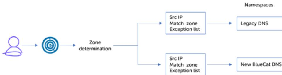
*This is typically the initial state when using BlueCat Edge with a traditional DNS migration*
