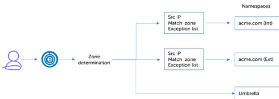
*This is the configuration that is used when having the same domain internally and externally. If the query is destined to the internet it is then forwarded to Cisco Umbrella*
