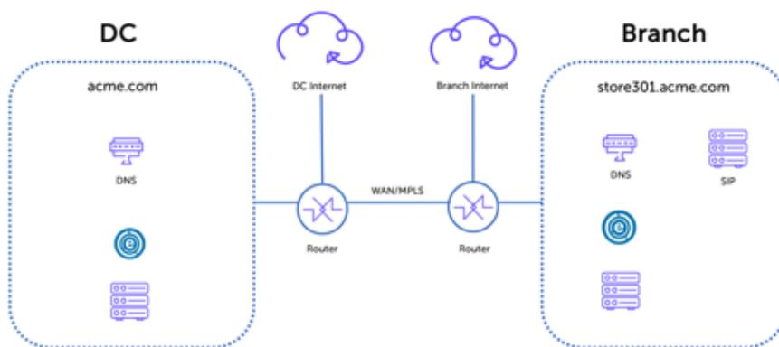
*Utilizing BlueCat Edge to provide local breakout to trusted services, while ensuring local resolution occurs properly.*
