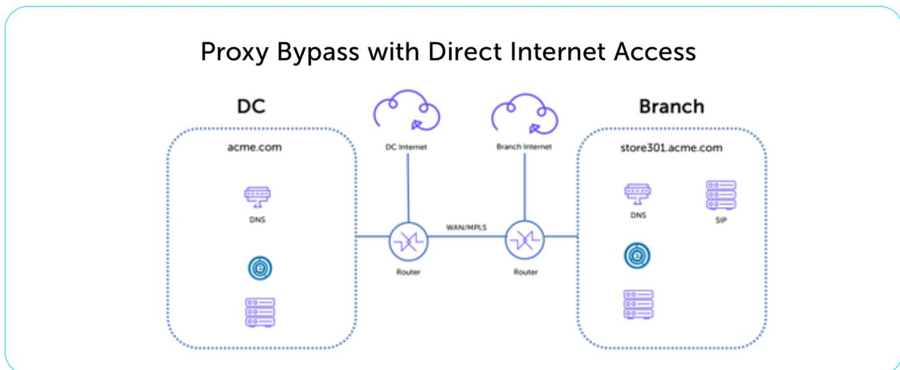
*Typical configuration for Proxy bypass with Direct Internet access from a remote branch.*
