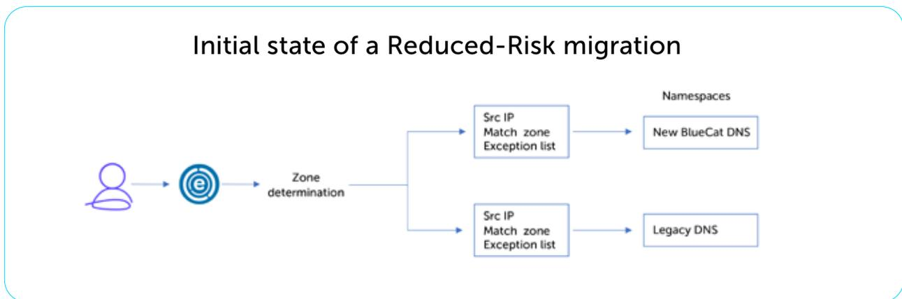
*This is typically the initial state when using BlueCat Edge with a traditional DNS migration*
