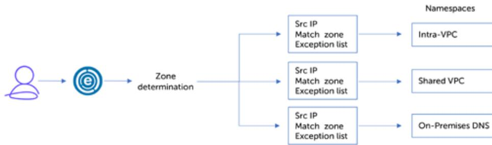
*This is typically the way that a cloud integration would be configured. Queries would go inside the VPC/VNET, then to a shared services VPC/VNET, then to the on-premises DNS.*
