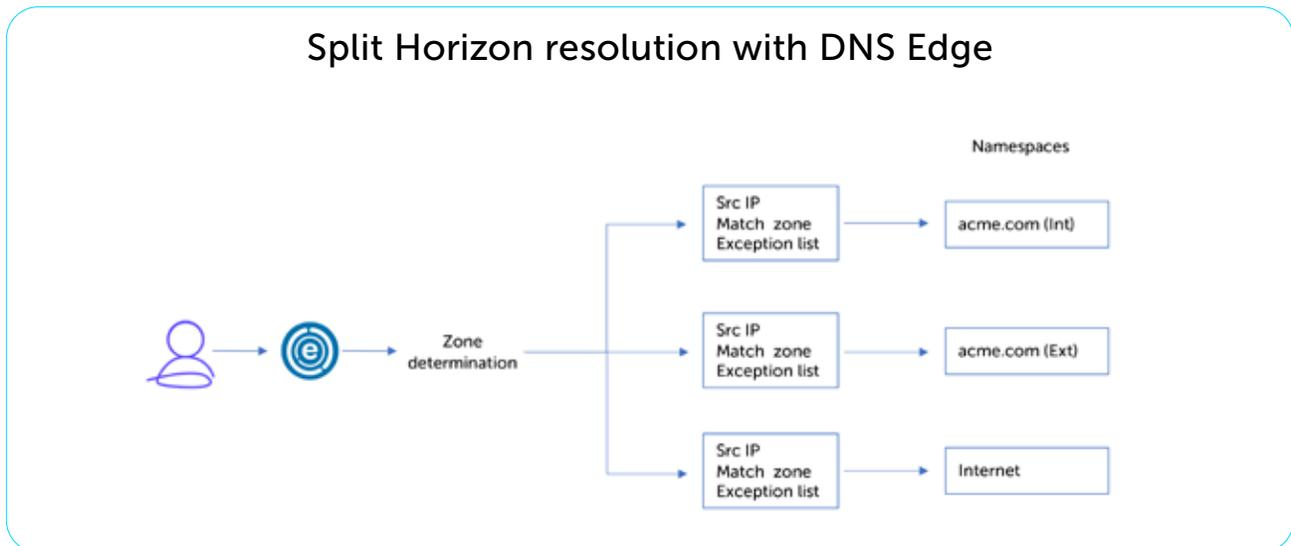
*When a customer has the same domain name internally and externally, oftentimes ensuring that the proper resolution path is utilized is the biggest challenge.*
